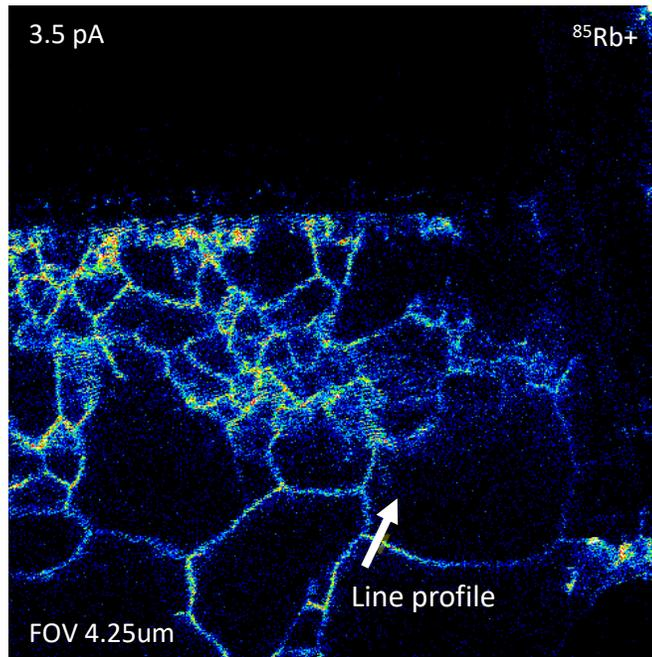
Apparent width of Rubidium signal between grains
