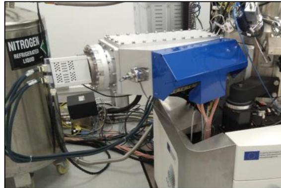
(Top) Photo of SIMS spectrometer (at LIST) and the continuous focal plane detector mounted to a vacuum flange.
