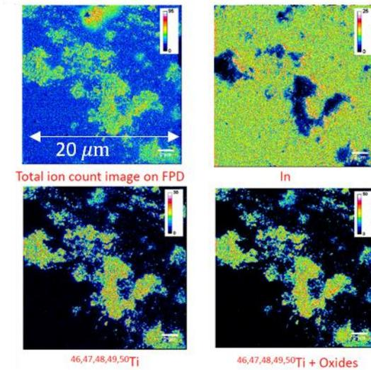
Data from by a continuous focal plane detector. Mass spectrum (Left) and surface compositional maps (Right). The sample under interrogation was titanium oxide nanoparticles on an indium phosphide substrate.
